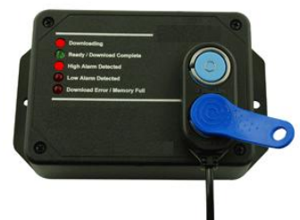
A simple and quick way to read the buttons without a PC . Plugged on an Ethernet port, it sends data from the button to Thermotrack-Webserve or Thermotrack-Online in less than 5 seconds.
