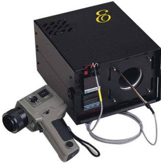
The Gemini R comprises a blackbody with which radiation pyrometers can be calibrated. The temperature of the cavity can be set to  $\pm 0.1^{\circ}\text{C}$  over the temperature range  $30^{\circ}\text{C}$  to  $55^{\circ}\text{C}$ . The temperature of the furnace is set on a controller, whilst an independent indicator, whose sensor fits into the cavity, indicates the actual radiance temperature. The sensor can be removed for external calibration or the complete system can be calibrated.
