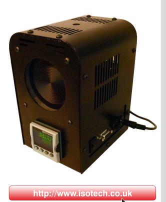
Response time is very fast, typically less than five minutes to achieve the required temperature (see graphs). The Model 989 can be used either horizontally or vertically.
